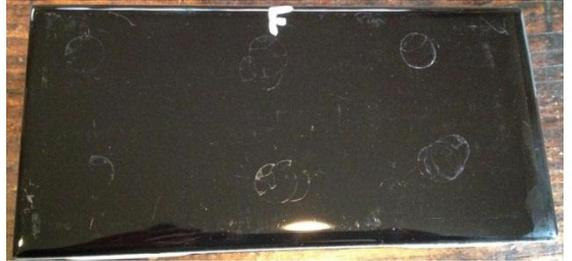
Spotting with Both Hardness and Silica Removed
